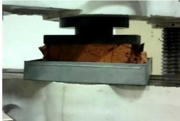
*Figure 4.1 Before Failure of brick*
