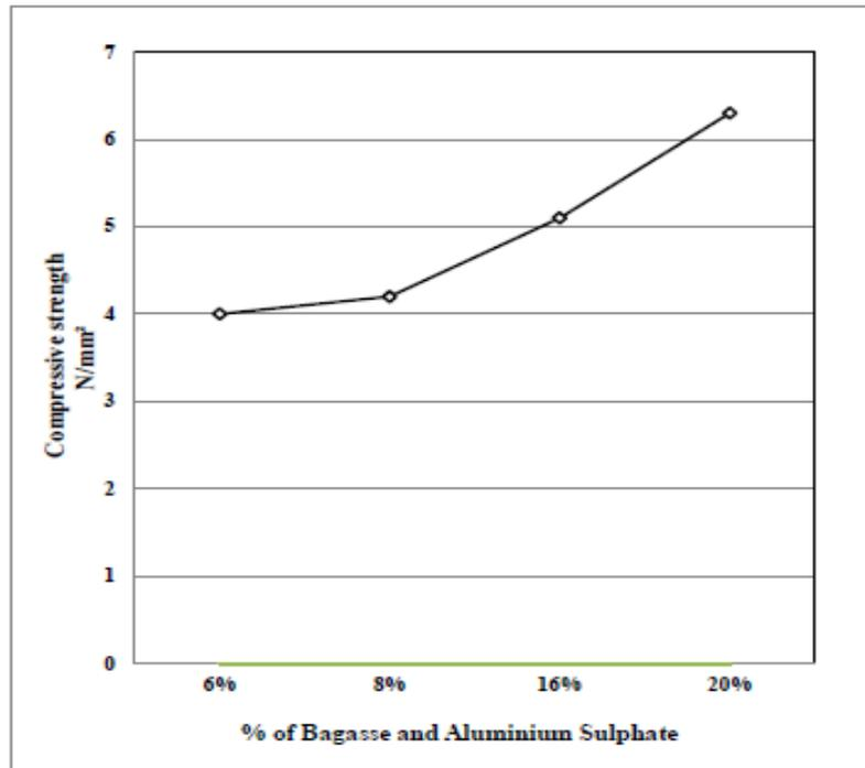
Figure 4.3: Compressive Strength of Bagasse ash Bricks.
